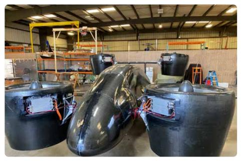
Sabrewing is preparing a prototype able to lift 1 ton of cargo for its official first flight this summer
