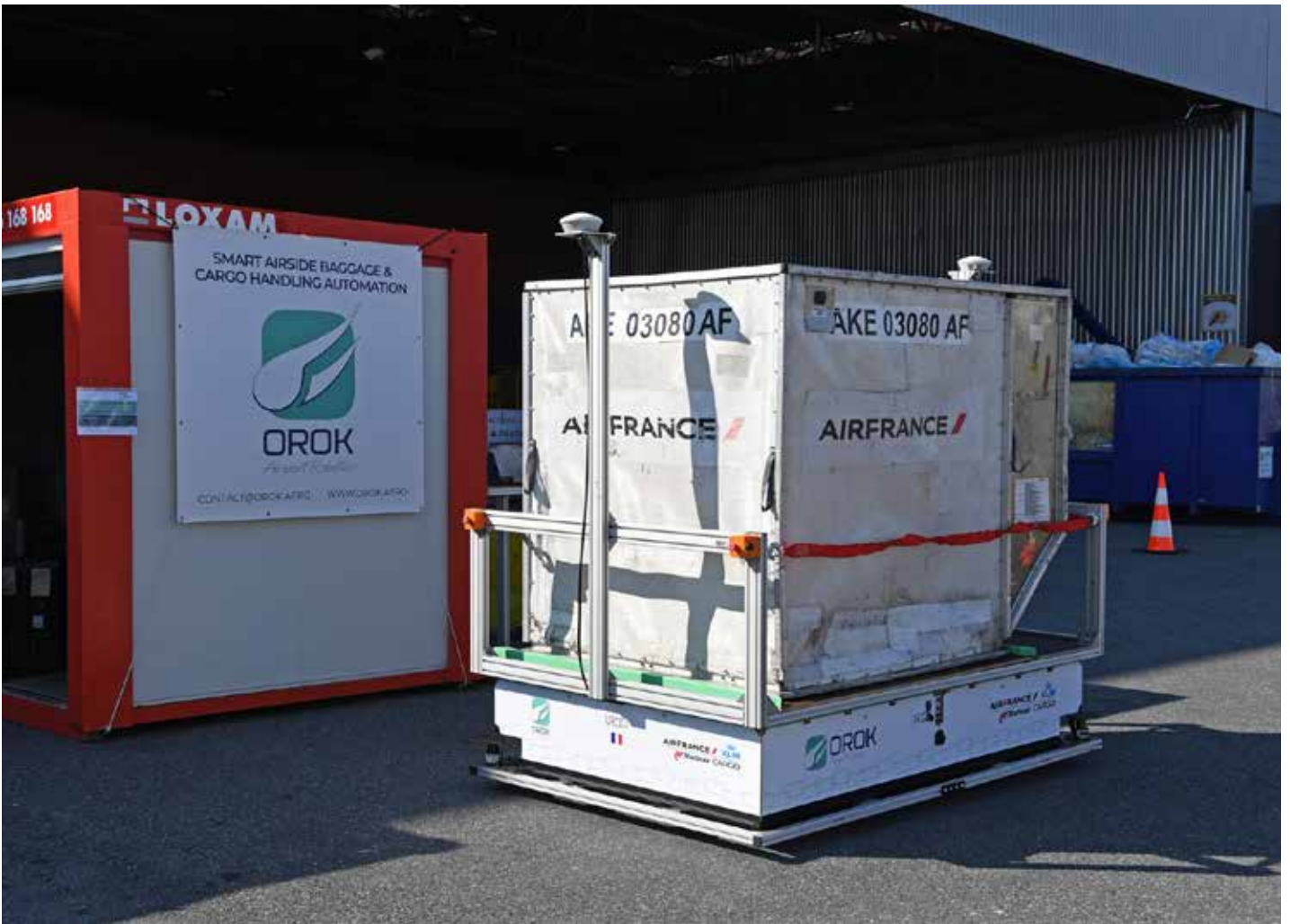
AF-KLM is testing an airside cargo transport solution at CDG using an autonomous electric vehicle
